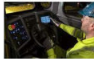
The optional cabin provides comfort to the operator with low noise level, air conditioner, spring suspended seat, information available in the display and controls within easy reach.
