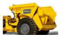
The optional Teletrain dump box releases material horizontally, making it the ideal choice for low ceilings.
